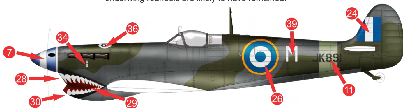
Spitfire Mk.Vc Trop., JK891, 335 Sqn. Arrived at Hassani from Italy on 16.11.1944 and was destroyed on 27.02.1945 during an emergency landing two miles southeast of the airfield. Finished in the type A day fighter scheme with sky tail band and a striped blue-white-blue Rotol Spinner. The camouflage colours were transposed, the dark green taking the place of the ocean grey in the pattern. National insignia were converted to Greek with the exception of the wing upper surface roundels which remained type IA as applied from January 1945. NOTE: Decal 35 is for the starboard side of the aircraft.
