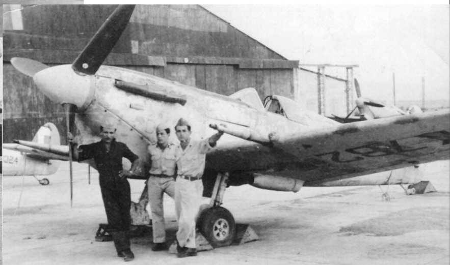
The photographs show JK782 near the end of its career, serving with the flight training school at Tatoi, near Athens in 1953. The overall silver finish is very worn, revealing the original colour as well as the original larger fuselage roundels. Phot.: Yiannis Gritsis collection via Tilemahos Panayiotides
